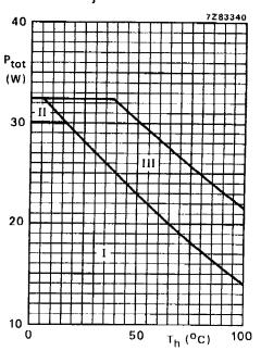
Fig. 3 Power derating curves vs. temperature. I Continuous d.c. operation II Continuous r.f. operation III Short-time operation during mismatch
