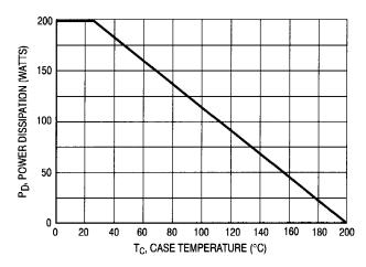
Figure 1. Power-Temperature Derating Curve
